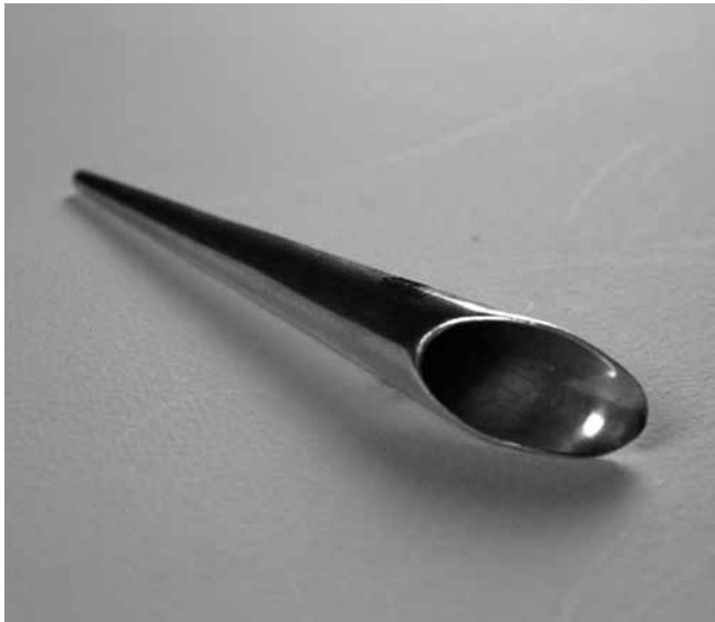
Fig 3: This contemporary silver zanshin has kept the 'arrowhead' of its classical antecedent but has been modified into a rounded conical shape. It is used for tapping and pressing.
