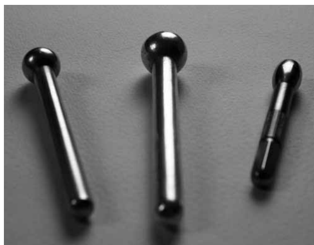
Fig 2: Enshin look like metallic lollipops and are used for very light rubbing of the channels.
